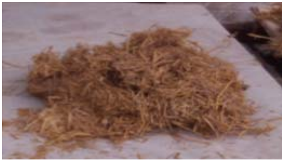
Fig. 1. Chipped rice straw fibre with 30 mm length
